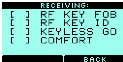
3. Press **OPEN** or **CLOSE** on key fob. After the signal is successfully received, you will see **[ + ]** in **RF KEY FOB** and **RF KEY ID**.
