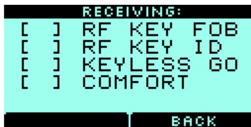
3. To receive the **RF KEY ID** signal, you must be at **up to 20 meters** from the car now when the key is brought to it. The car's mirrors will open and **[ + ] RF KEY ID** will appear on the device screen.
