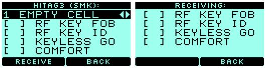
3. Press **OPEN** or **CLOSE** on key fob. After the signal is successfully received, you will see [+] in RF **KEY FOB** and **RF KEY ID**.
